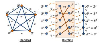
**Figure 1.** *Illustration of the standard and the bijection* ALLDIFFERENT *encodings*. In the bijection encoding, a 1-to-1 mapping of the bit-vectors is found first. Then the values of bit-vectors are forced to be linearly ordered according to their position in the mapping.
